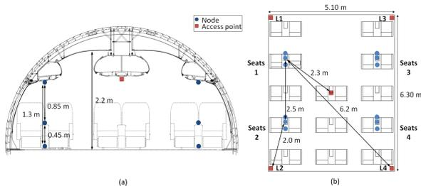
Figure 2: Sensors deployment, a) cross-section and b) top-level view.
