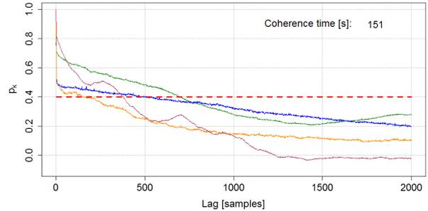
Figure 4: Coherence time analysis for different cabin locations (seats).
