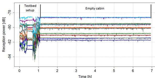
Figure 3: RSSI traces of all WSNs to one WDC, showing multiple reception power levels, caused by dynamic and static shadow fading.
