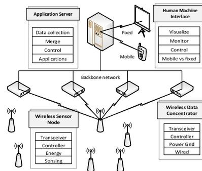
Figure 1: System components overview and their interaction.
