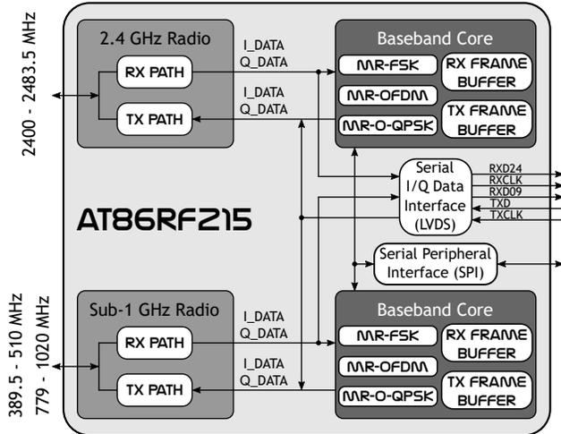
Figure 2. AT86RF215 block diagram.
