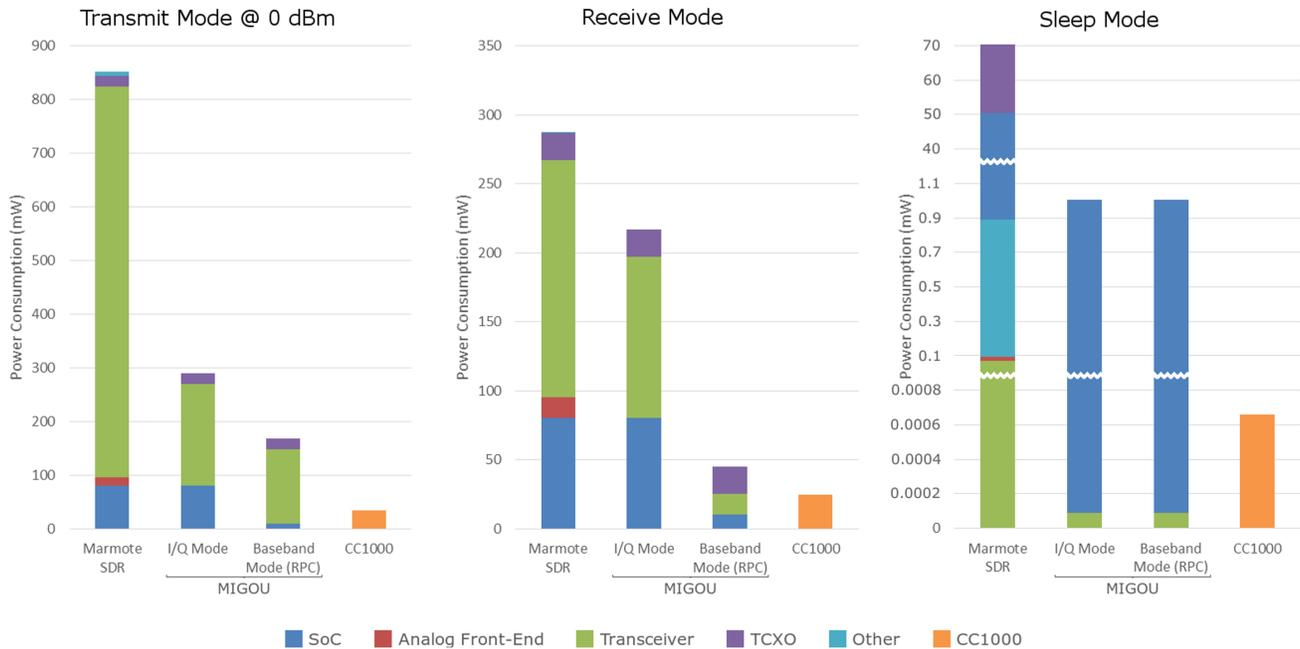
**Figure 4. Power consumption comparison in milliwatts (mW).**
