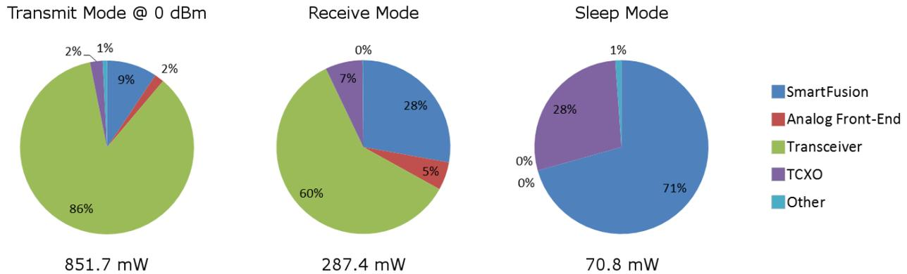
**Figure 1. Power consumption of the MarmotE SDR platform in various operation modes.**
